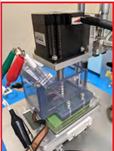
CMP Head with rotational motor and polishing Pad
